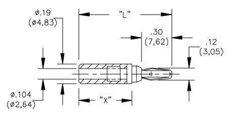
Model 3690 "X" = (11,43mm) 0.45" "L" = (22,61mm) 0.89" Model 4617 "X" = (25,40mm) 1.00" "L" = (36,32mm) 1.43"
