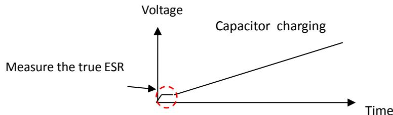
Using 4 wire measuring, make sure the meter can measure the capacitor with low noise.
